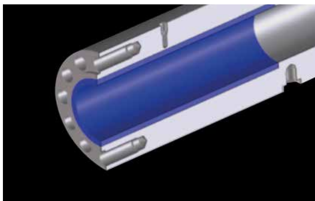
Repair by fitting a liner
